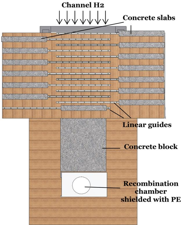
Fig. 2 Top view of the research stand with mounted linear guides, concrete block and shielded recombination chamber
